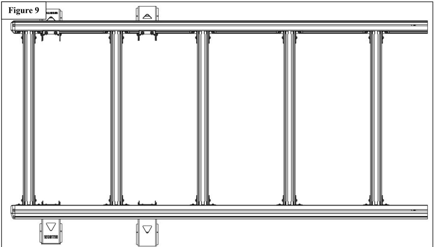
9. Add one M6 Slide Nut on both Driver and Passenger Rail Rack (**Item 8 & 9**) on the Upper Top Groove. See **Figure 3** for reference.
