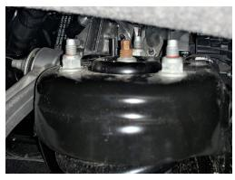
27. Place the lower strut mount onto the lower control arm. Torque the original lower strut bolts and nuts to 66 ft lbs.
