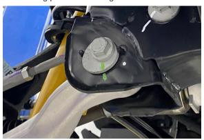
10. Remove the two lower strut 18mm nuts and lower end link 21mm nut on the control arm. If the end link ball joint turns, use a hex key to prevent the stud from turning while removing the nuts.
