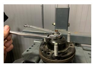
17. Detach the upper spring isolator from the top mount. If needed, use a pry tool or flathead screwdriver.
