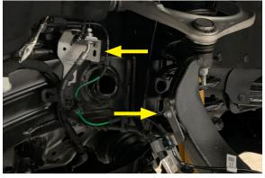
11. Remove the steering tie rod end nut with a 21mm socket from the spindle. Use a tie rod end remover to carefully detach the tie rod end from the spindle. Alternatively you can strike the spindle with a hammer to remove the tie rod end. Do not hit the boot.
