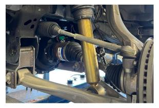
33. Reattach the sway bar end links to the lower control arm, torque to 111 ft lbs.
