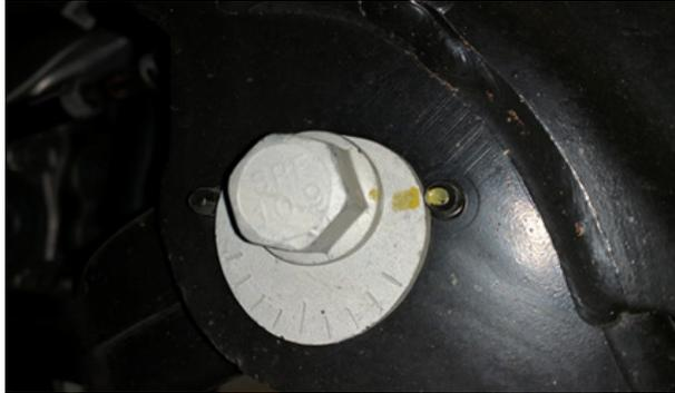
11. Working on one side at a time, loosen and remove the crossmember bolts that connect the lower control arm and frame.
