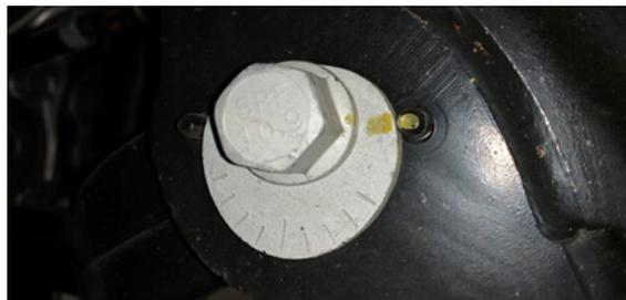
33. Reinstall the sway bar. The bushing bracket will be torqued to 66 lb.ft and the end link nuts will be torqued to 111 ft-lbs.
