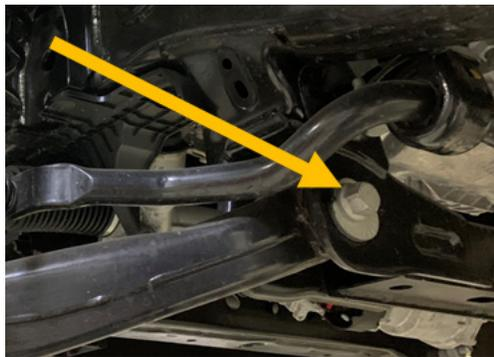
32. Set the alignment settings to the markings made before installation.
