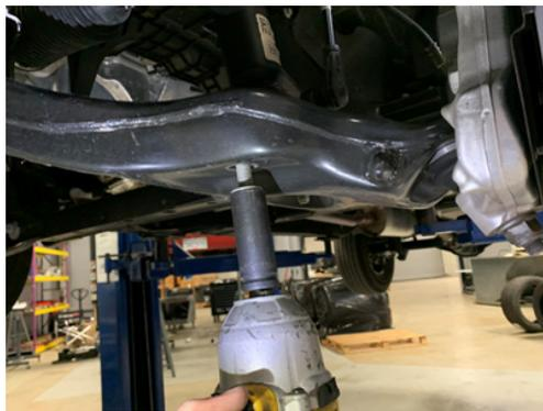
31. Reattach the lower control arm to the frame using the OE alignment hardware. Do not tighten or torque until your vehicle is back on the ground. Torque to 210 ft-lbs.
