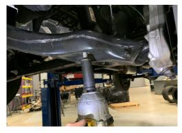
13. Push the spindle and lower control arm down and back until the lower shock studs are clear of the control arm.
