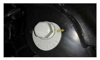
11. Working on one side at a time, loosen and remove the crossmember bolts that connect the lower control arm and frame.
