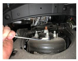
30. Attach the lower coilover mount to the lower control arm using the supplied bolts and Nylock nuts. Torque the supplied nuts to 66 ft-lbs.
