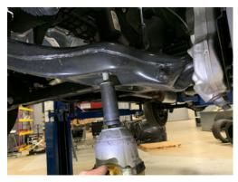
31. Reattach the lower control arm to the frame using the OE alignment hardware. Do not tighten or torque until your vehicle is back on the ground. Torque to 210 ft-lbs.
