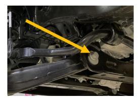
12. Loosen and remove the nuts securing the lower strut mount to the control arm.
