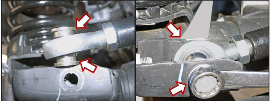
Fully tighten all OEM hardware at upper frame mount & axle mount. Fully tighten jam nut of Skyjacker adjustable front track bar using a 1-1/8" wrench.
