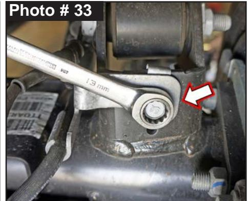
16. Connect OEM rear brake line brackets to rear differential with OEM hardware using a 13mm socket / wrench. (See Photo # 33)
