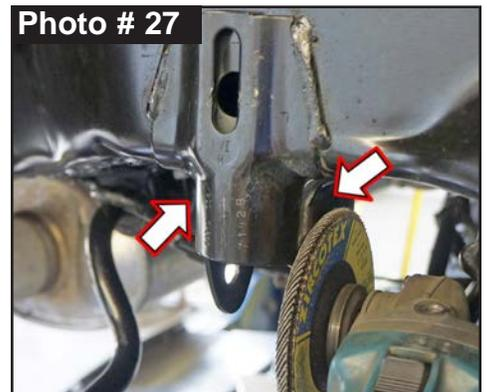
10. Install Skyjacker # JLRTBU-B Rear Track Bar Upper Bracket over OEM rear upper track bar bracket on frame.
