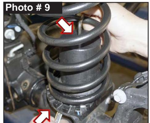
16. Raise front axle in order to load Skyjacker front coil springs. **Note:** There has been occasional reports of Passenger Side coil spring having an inward bow after installation on taller lifts. If so, OEM upper coil spring isolator can be rotated 180 degrees.
