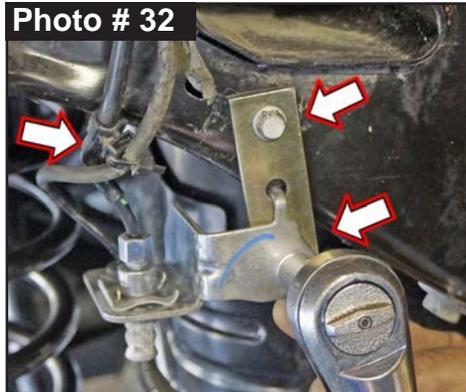
Slightly bend \ straighten OEM rear hard brake line. **Note:** Be very careful not to damage OEM rear hard brake lines.
