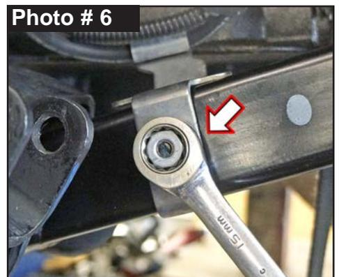
10. Mark the location of OEM front driveshaft\flange at axle & disconnect using a 15mm socket \wrench. (See Photo # 7)
