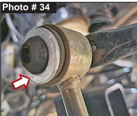
Attach lower end link with OEM hardware with large washer to bushing side of end link using a 18mm socket \ wrench. (See Photo # 35) Secure, but Do Not Completely at this time.
