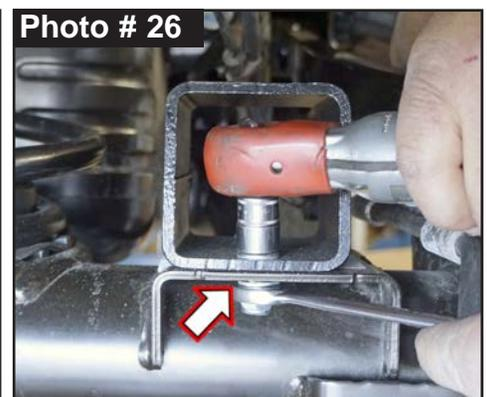
9. Check fit Skyjacker # JLRTBU-B Rear Track Bar Upper Bracket over OEM rear upper track bar mount on frame. The double hole side of Skyjacker track bar bracket towards outside of vehicle. (See Photo # 28)
