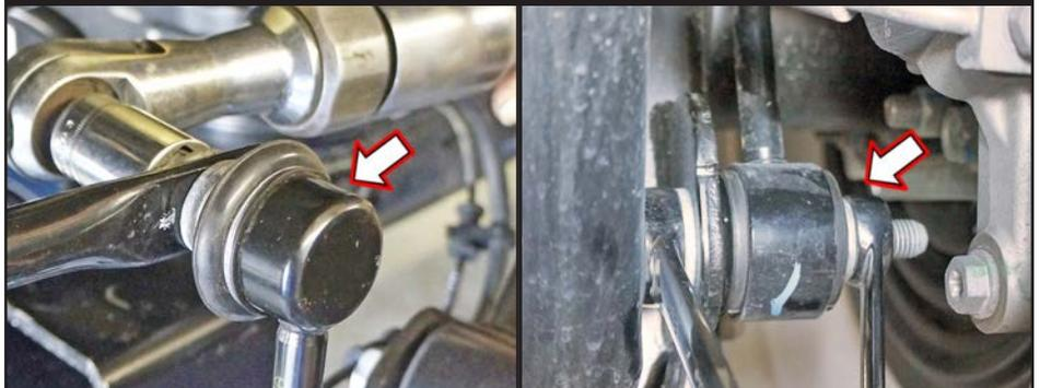
4. Disconnect OEM rear brake line brackets from frame using a 10mm socket \ wrench. (See Photo #21) Disconnect OEM rear brake line brackets from rear axle at upper control arm mount using a 13mm socket \ wrench. (See Photo #22)
