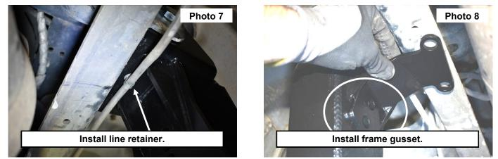
frame gusset and the bottom of the frame are flush with one another, Torque to 120ft-lbs, using a 22mm socket and wrench. See Photo 9.
