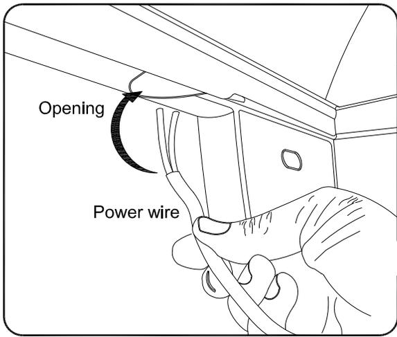
Feed end of power wire through opening on drivers side of truck cap, then down through the side panel to the ground. Leave 2' of power wire in the truck bed.
