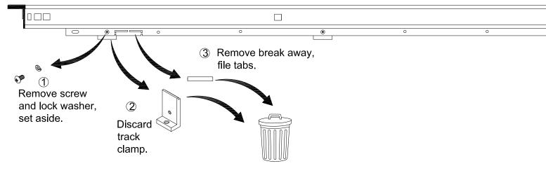
Key supplied track clamp bracket  $\overline{\mathbb{Z}}$  onto the back of the track at the slotted hole. Using the same screw and washer that was removed loosely attach bracket to track.
