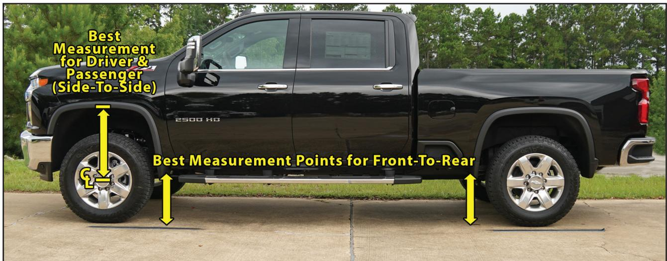
**FINAL CHECKS****6) CLEARANCE CHECK...**
