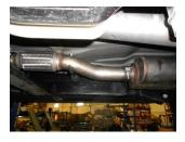
5) Place the provided 3" clamp onto the inlet of muffler #853057-Z, then connect the inlet of the muffler to the inlet pipe and support with a stand. Tighten the clamp just enough to hold in position.
