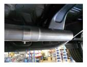
2) If installing the system on a Crew Cab truck with a 6.5' bed, place extension pipe **#TB700S** onto the back of the **#26401S** inlet pipe, place a provided clamp onto the slip-fit and tighten enough told hold in position. The extension pipe will not be used on Double Cab-6.5' bed or Crew Cab-5.5' bed models.
