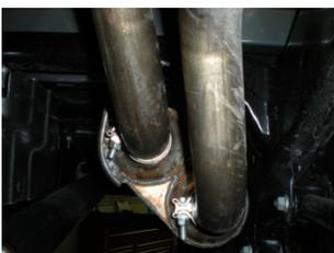
4) Place the provided 2 1/4" clamps onto the muffler outlets and re-install the tailpipes into the muffler outlets. Be sure to line up the tabs on the tailpipes with the notches on the muffler outlets. Tighten the clamp securely.
