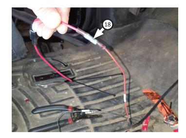
20. Place wire tap (19) onto fuse holder then close them around blue socket wire. Pinch fuse holder to splice fuse wire in with socket wire, then close fuse holder to encase connection.
