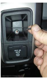
15. Pull center console front off of dashboard just enough to gain access behind it. Leave all wiring attached.
