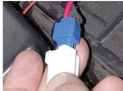
21. Open fuse holder cap, plug in **micro fuse (17)**, then replace cap.
