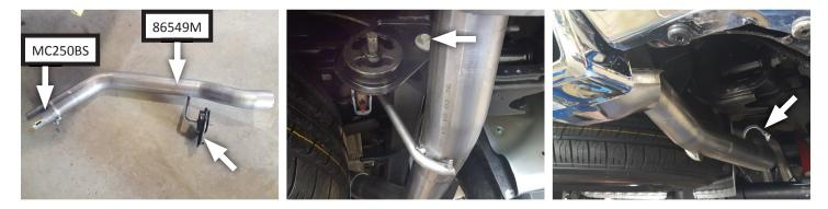
15. Place **clamp (MC250BS)** and mount (removed step 4) onto **left rear tailpipe (86548M)** then connect it to left front tailpipe. Bolt mount onto frame then tighten clamp enough to allow for adjustment.
