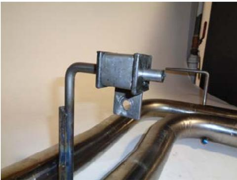
4) Place the supplied **HA602** rubber hanger onto the wire hanger closest to the tips of exit pipe assembly **#86463M**.
