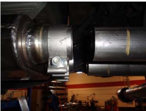
5) Place a supplied 2 ½" clamp over each muffler outlet; then place exit pipe assembly **#86463M** into the back of the muffler approximately 2". Connect the wire hanger closest to the muffler to the rubber mount on the vehicle. Tighten the clamps at the muffler outlet enough to hold but still allow for adjustment.
