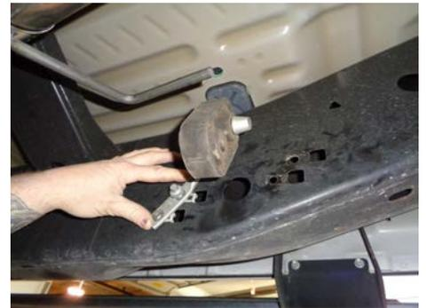
4) On some vehicles the front frame mount may be in the incorrect location to properly connect to the 490HA frame hanger. In this case, remove the two screws attaching the mount to the frame, move the two plate nuts to the forward set of holes and remount the hanger to the frame.
