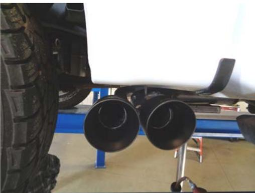
9) Adjust the position of all pipes and muffler to provide a satisfactory fit. A minimum 3/4" clearance around all parts of the system must be maintained; while also keeping suspension travel and vibration in mind.
