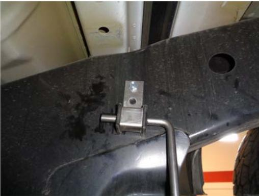
8) Adjust the exit pipe so that the tips are the desired distance from the body, then rotate the **HA572** hanger so that it lays flat against the inside of the vehicle frame and use a center punch to mark the center of the two holes on the frame. Rotate the hanger out of the way and drill each mark using a 1/4" drill bit. Use the two 5/16" thread cutting bolts to secure the hanger to the frame. Tighten securely.
