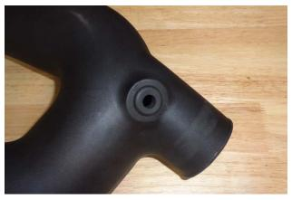
13. Install grommet (15) in intake tube (12). (Moistening the hole with soapy water will ease insertion.)
