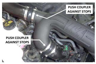
18. Push each coupler up against its stops on the turbo duct and tighten its turbo duct clamp. Center the intake tube between all the couplers, so that there are approximately equal amounts of tube inserted in each coupler. Then tighten the three screw clamps on the intake tube.
