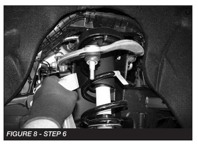
Locate the plastic wire harness channel on the top of the passenger side coilover mount. Push it up and back to allow access to the three coilover nuts. Remove and discard the upper coilover nuts. SEE FIGURES 9-10
