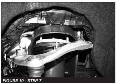
Remove and save the two lower coilover bolts. Then remove the coilover assembly from the vehicle. SEE FIGURES 11-12
