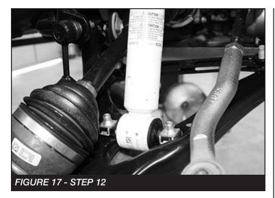
Locate the factory bumpstop tab on the frame mount.
