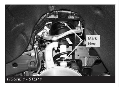
Starting with the passenger side. Disconnect the ABS wire bracket from the upper control arm and the brake line bracket from the knuckle. Save hardware. SEE FIGURES 2-3
