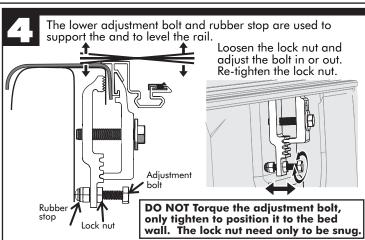
Repeat all of the steps for both sides. Return to the standard installation instructions. Follow step 2 for the bulkhead seal, then skip to step 8.
