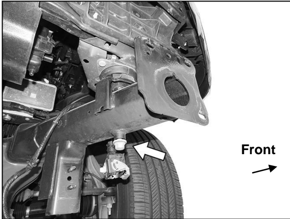
(Fig 5) Models without tow hooks, loosen but Do Not Remove body bolt (arrow)
