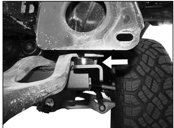
(Fig 10) Models with tow hooks, insert 1/2" Thin Spacer between tow hook and top of Bracket (arrow)
