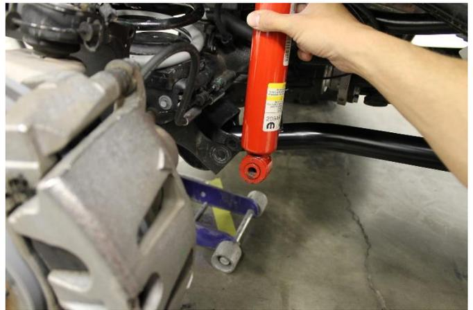
9. Raise Vehicle frame and/or lower front axle to remove coil spring
