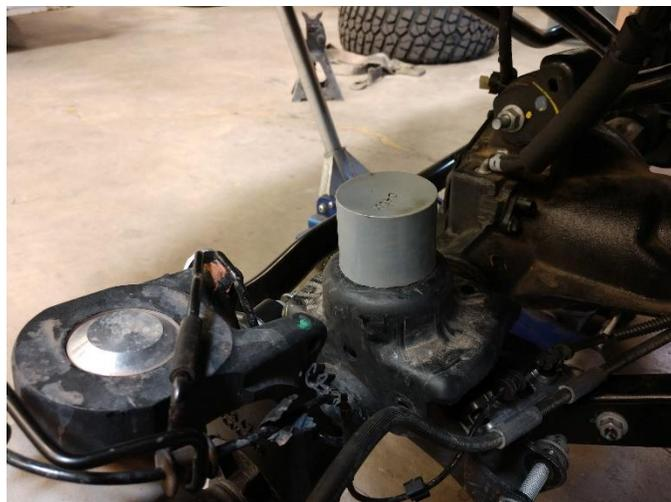
11. Install Daystar front driver side coil spring corrector (Part Number: 07005)
