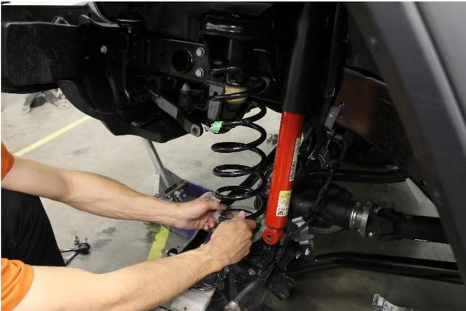
10. Remove bottom coil spring isolator
