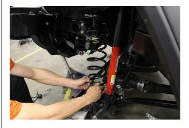
9. Remove bottom coil spring isolator
