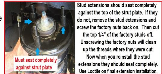
Stud extensions should seat completely against the top of the strut plate. If they do not, remove the stud extensions and screw the factory nuts back on. Then cut the top 1/4" of the factory studs off. Unscrewing the factory nuts will clean up the threads where they were cut. Now when you reinstall the stud extensions they should seat completely. Use Loctite on final extension installation.
