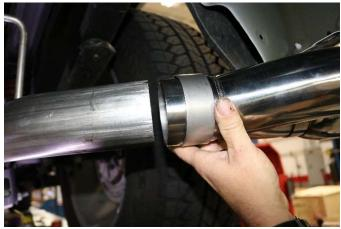
**15.** Slide the expanded and notched end of the 4" Pro Series Tip Assembly into the rear section of the TailPipe Assembly as shown.
