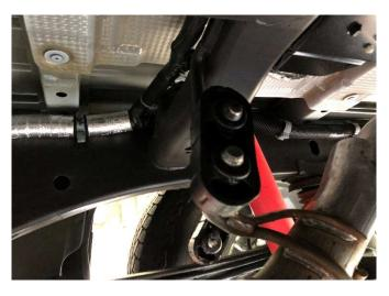
**5.** Remove the left grommet from the left tailpipe hanger at the muffler exit, using grommet pullers or similar device.
