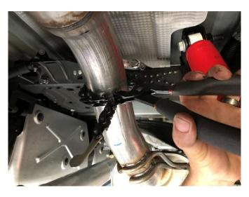
1. Scribe a line 6" from the hanger next to the muffler closest to the rear of the vehicle.
