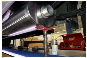
**6.** Use a stand to support the other end of the muffler as shown.
