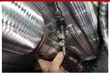
**3.** Insert the spherical clamp into the factory pipe as shown. Make sure that the pipe is fully seated in the connection. Snug the spherical clamp using a 13mm socket.
