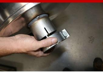
**4.** Put the 3" TORCA clamp on the expanded and notched end of the muffler.
