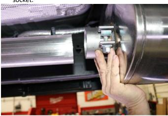
**5.** Slide the expanded end of the muffler into the headpipe.
