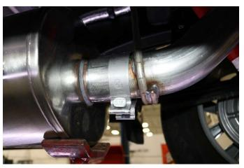
**9.** Slide the TailPipe Assembly into the side of the muffler supported by the stand as shown.
