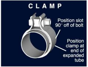
**NOTE:** Align all clamps so that the center of the clamp bolt is 90 degrees from the notch in the pipe.
