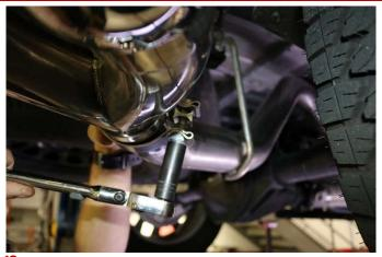
**16.** Snug the TORCA 3" Clamp on the tip assembly using a 15mm socket.
