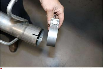
**8.** Insert a 3" TORCA clamp into the expanded and notched end of the TailPipe Assembly as shown.
