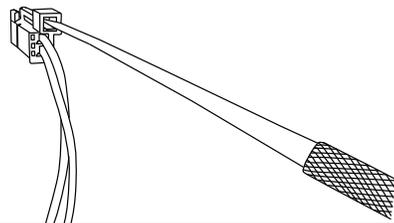
14 **Note:** It's best to reach from both sides when installing 2 pin plug. Use bottom left port as shown.
