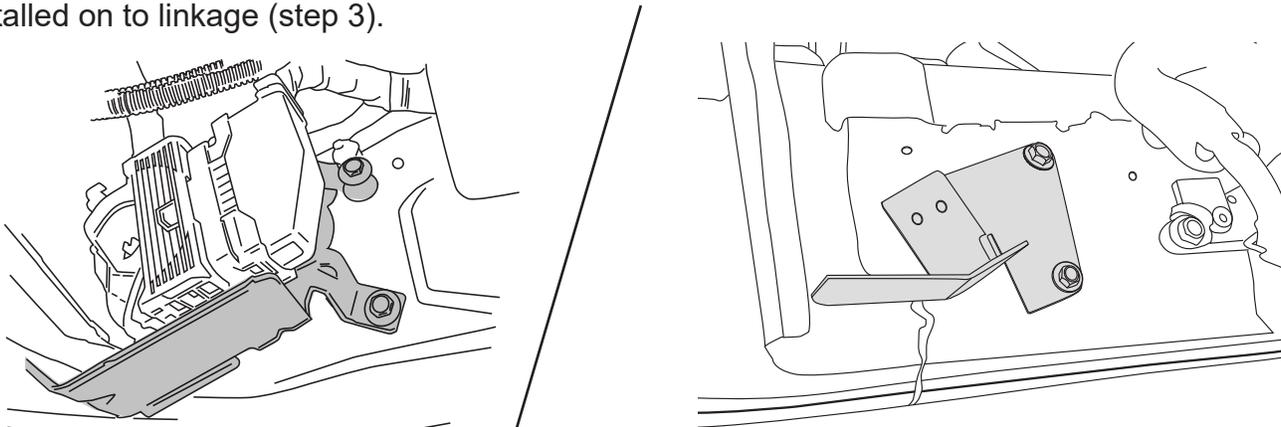
Locate mounting points. First and last set of studs on the inner sill. Motor linkage mounts towards the front of the truck and Idler towards the rear. Driver side shown below.
