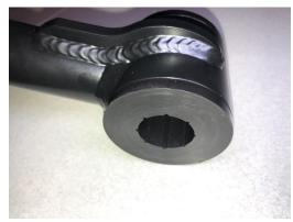
O. Apply the supplied grease to the bushing inside diameter.
