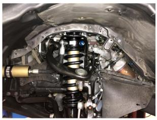
G. Using two 19mm wrenches, remove the nut and washer securing the UCA bolt.
