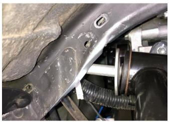
Carefully remove the UCA bolt. The UCA can now be removed. Save the UCA bolt and flanged nut as they will be reused later. The OE washers can be discarded.
