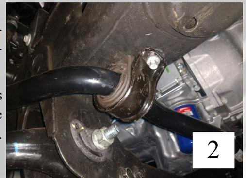
**The bar should be installed so that the ends pass ABOVE the lower control arms. Shift the bar side to side and front to back to center on the chassis . Be cautious not to damage brake lines while installing the Belltech Anti-Sway bar.**
