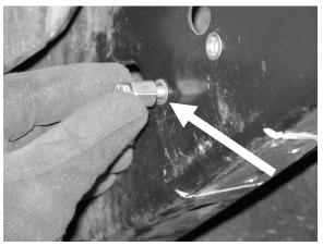
**STEP 1G:** To lock the nut-sert in place in the chassis tube frame, using a 7/16" wrench or a ratchet with a 7/16 socket head (bolt) and a 1/2 wrench (nut sleeve), begin tightening the bolt. The knurl end of the nut-sert locks into the thickness of the chassis tube frame, while the end expands on the inside. Tighten until you are not able to turn it anymore, just stopping short of not being able to turning it. Do this for all three holes that have been just drilled.
