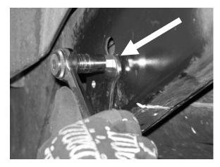
**STEP 1H:** Remove all three mounting bolts (1/4-25 x 1") that were just used to mount the nut-serts. Remount the END LINK BRACKET, tightening all three mounting bolts. WE RECOMMEND mounting all three mounting bolts at this stage.
