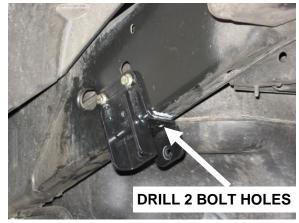
**STEP 2B:** Remove the END LINK BRACKET
