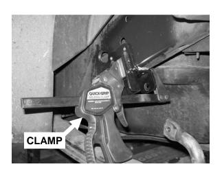
**STEP 1D:** Using a 9/32 drill bit, and with the END LINK BRACKET clamped in place, drill the three (3) clearance holes into the chassis tube frame.
