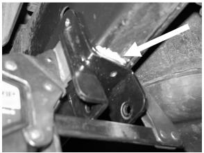
STEP 1B: With a cleaning solvent, clean the area where the END LINK BRACKET will be located.
