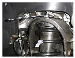
26. Attach the lower strut mount to the lower control arm with the two OEM bolts and torque to 37 ft lbs.
