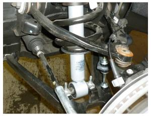
27. Reattach the end links to the lower control arm and sway bar. Torque the sway bar end link nuts to 17 ft lbs. when the vehicle is back on the ground or the suspension is loaded.
