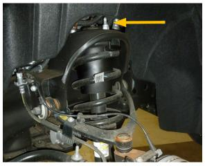
11. Remove the two lower strut mount 15mm bolts.
