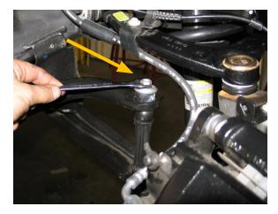
10. Locate the three top studs on the front strut assembly and remove all three mounting 18mm nuts.
