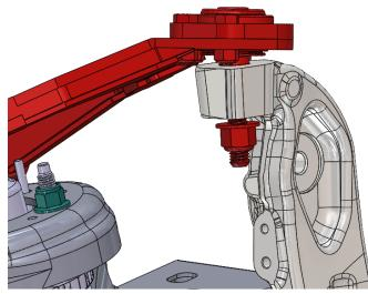
11. Insert the upper ball joint into the spindle. A pry bar may help to pull the arm down into position. Torque to spec
