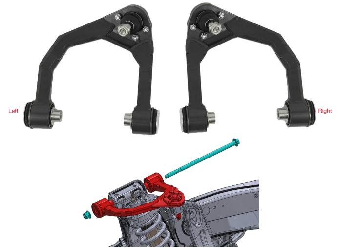
10. While holding the arm up so the top of the ball joint sits level to the ground, torque the mounting bolt to oe spec.
