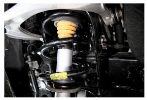
26. Attach the lower strut mount to the lower control arm with the two OEM bolts and torque to 37 ft lbs.
