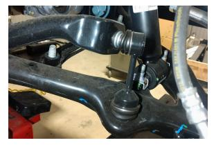
12. Push or pry down on the lower control arm to gain clearance and remove the strut.
