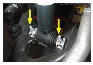
11. Remove the mounting nut holding the anti-sway bar end link to the lower control arm. The nut is located on the underside of the lower control arm. This will allow the lower control arm to swing down and ease the removal of the strut.
