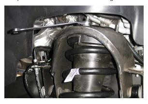
10. Remove the bottom bolts on the OE strut and lower control arm using a 15mm wrench.
