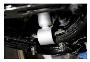
27. Attach the end link to the lower control arm, torque to 74 ft lbs. when the suspension is loaded or the vehicle is back on the ground.
