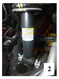
2d. Remove the mount nuts from the end links. Detach the sway bar from the end link. (**Photo 3**)
