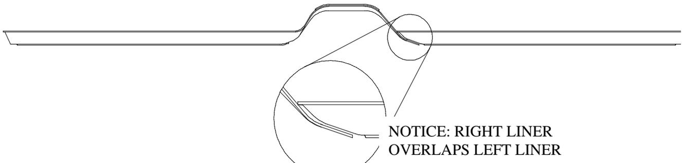
TUNDRA OWNERS WITH THE POWER SEAT OPTION WILL NEED TO TRIM THEIR DRIVER'S SIDE LINER TO ALLOW CLEARANCE OF THE POWER SEAT TRACK (SEE ABOVE). REMOVE THE MATERIAL FROM THE TWO RAISED AREAS. A UTILITY KNIFE OR SCISSORS WORK WELL.
