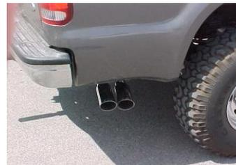
INSTALL YOUR STAINLESS TIPS. TIGHTEN ALL CLAMPS STARTING FROM THE FRONT, WORKING YOUR WAY TO THE BACK OF THE TRUCK. TO CLEAN TIPS USE A STAINLESS STEEL CLEANER & SCOTCH BIE PAD.
