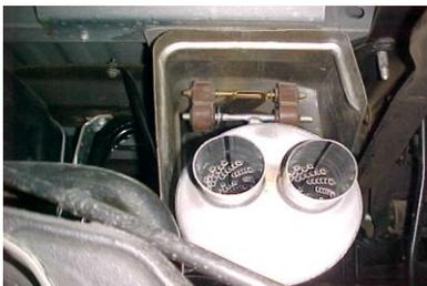
SLIP MUFFLER # B THROUGH BAND CLAMP THEN ONTO THE HEADPIPE 1 1/2" TO 2". THE OUTLETS WILL BE ON THE TOP. USE CLAMP # F TO SECURE MUFFLER TO HEADPIPE. DO NOT TIGHTEN.
