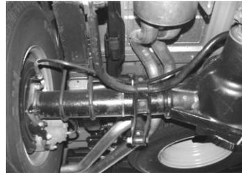
INSTALL DRIVER SIDE OVER AXLE TAILPIPE # D INTO MUFFLER 1 1/2 TO 2". INSERT WELDED HANGER INTO RUBBER GROMMET, USE CLAMP # G TO SECURE PIPE TO MUFFLER. THIS PIPE WILL GO INTO THE DRIVERS SIDE OUTLET. DO NOT TIGHTEN
