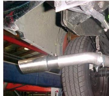
CUT 5 INCHES OFF EACH EXIT PIPE, THEN INTSTALL EXIT PIPES # F TO THE OVERAXLE TAILPIPES, USE CLAMP #G TO SECURE. USE ZIP TIES FOR BRAKE AND HOSE LINES TO KEEP AWAY FROM PIPES. NOW FIRMLY TIGHTEN ALL BOLTS, CLAMPS AND HANGERS. INSTALL YOUR STAINLESS TIPS TO YOUR DESIRED LOOK.
