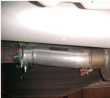
INSTALL MUFFLER ONTO HEADPIPE AT LEAST 1.5" TO 2", AND ATTACH USING CLAMP #H.. USE A JACKSTAND TO SUPPORT THE MUFFLER. DO NOT TIGHTEN.
