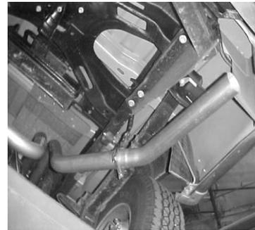
INSTALL PASSENGER OVERAXLE TAILPIPE TO THE OUTLET OF THE MUFFLER 1.5" TO 2". THE TAILPIPE INLET THAT GOES INTO THE MUFFLER IS 4.5" LONG AND ATTACH WITH CLAMP # G. DO NOT TIGHTEN. INSERT WELDED HANGER INTO RUBBER GROMMET.
