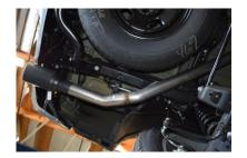
Install the Gibson Tips onto your exit pipes. Place the tips to your desired position. Be for tightening down the system it is recommended to secure the tips in the position you want and check the location after each connection is tightened.
