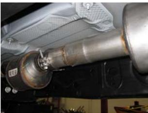
3. Install the muffler assembly onto the factory dome 2". Use a jack stand to support the muffler assembly. Use your factory clamp to secure muffler assembly to the dome. Do not tighten. Insert welded hangers into rubber grommets.
