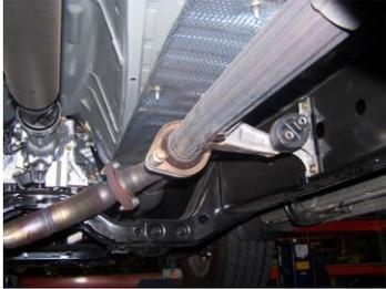
Lay out the exhaust on the floor so it looks like the drawing and compare parts with manual. **To remove the stock exhaust remove, it from the 2-bolt flange, just in front of the muffler.** Then cut your tailpipe off behind your factory muffler.
