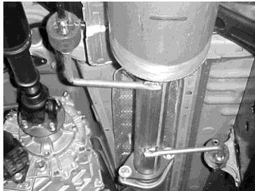
Install head pipe # A on to your existing stock 2 bolt flange. Use hardware kit #G, to secure. **DO NOT TIGHTEN.** Insert welded hanger into rubber grommet.
