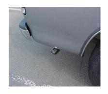
NOW INSTALL THE STAINLESS STEEL TIP USE ANY ALUMINUM OR STAINLESS STEEL CLEANER TO POLISH YOUR TIP. TIGHTEN ALL CLAMPS AND HANGERS STARTING FROM THE HEADPIPE BACK
